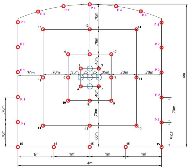
Figure 2. Firing sequence (4 m x 4 m). NONEL + EZshot used in limestone.
